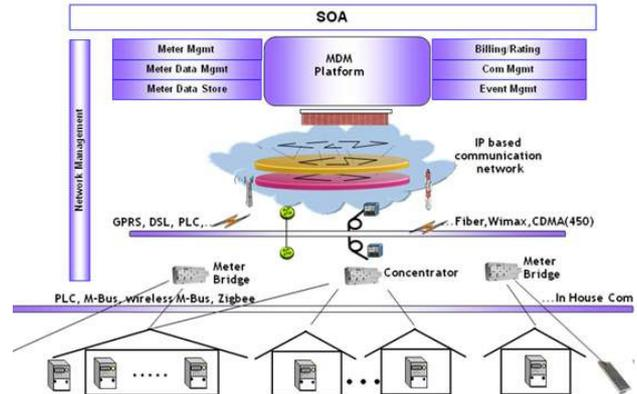
Figure 6. Layered Generic Communication Architecture
