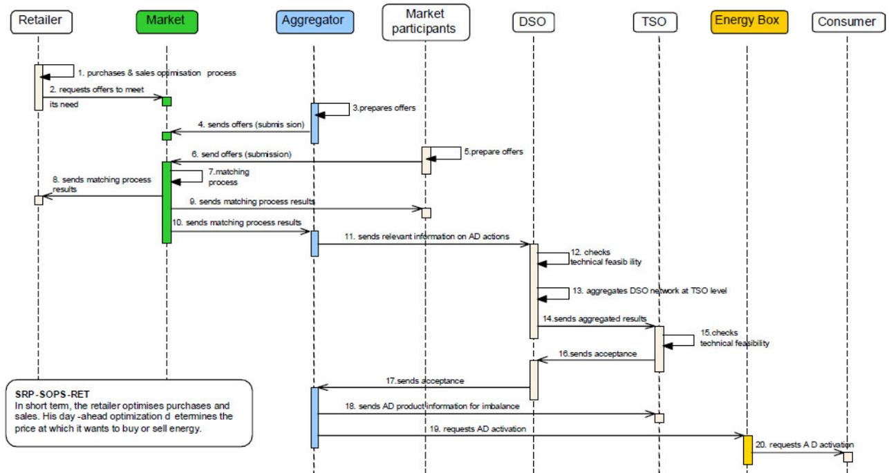
Figure 1. ADDRESS Service Sequence Diagram Sample [SRP-SOPS-RET], see [3] for further details
